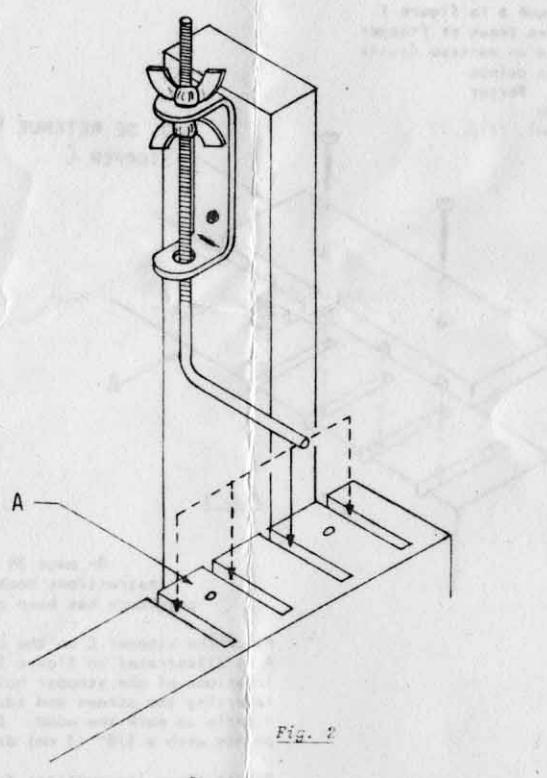
Install the batten swords on top of the loom by inserting the L-shaped rod into one of the four notches of cross-members A and B. (Fig. 2)
