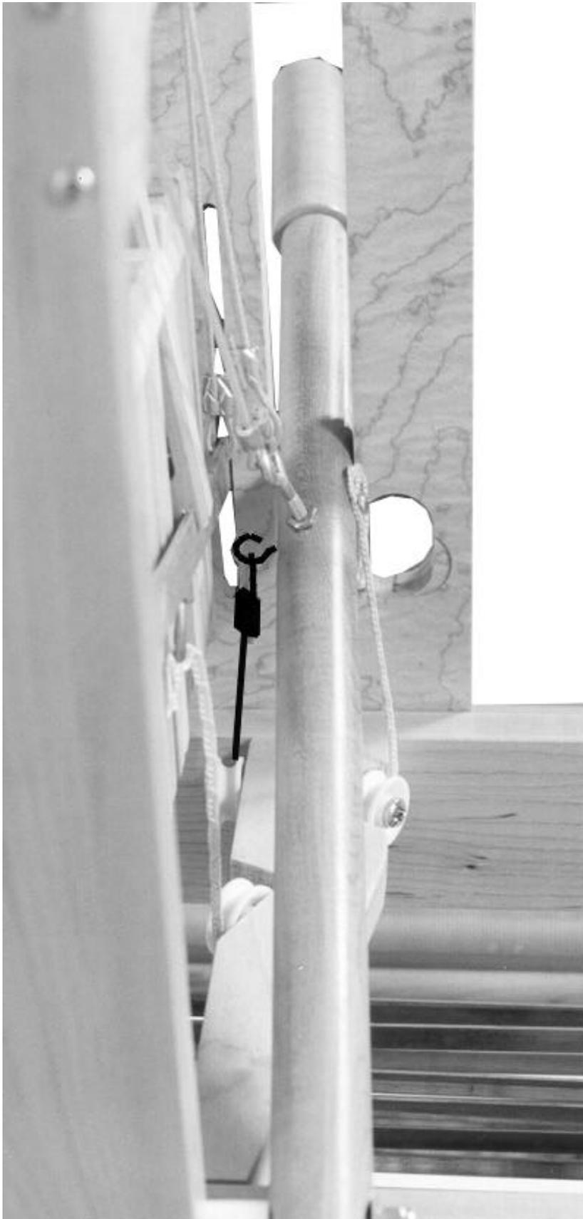
Install metal wire joining the screw hook of right treadle and screw hook at the back of the handle.
