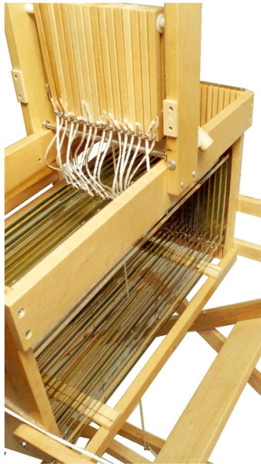
All loop cord should be now under tension (weight of the shaft frame) and loop cord should pass outside of the gold metal rod.
