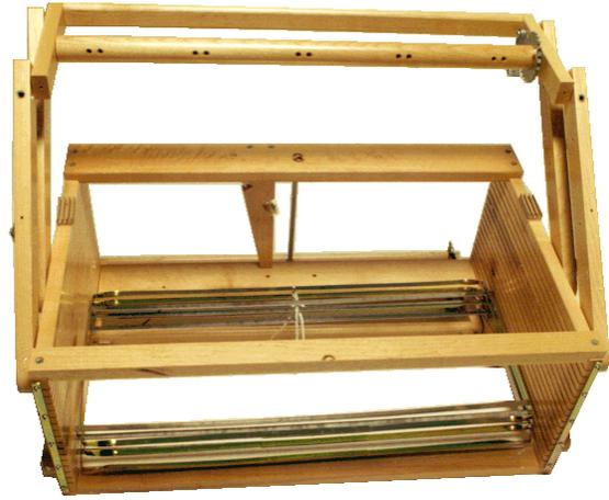
**When all the 16 shaft frames are installed and before you move the loom, put the 2 soft wood board (with black mark) under the shafts so they will not slide out of the castle frame.**
