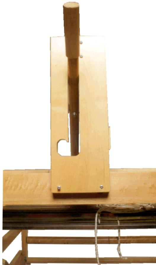
Make connection of the loop cord between the knife and the handle outside screw at black mark. Pass hole of black mark around the screw.
