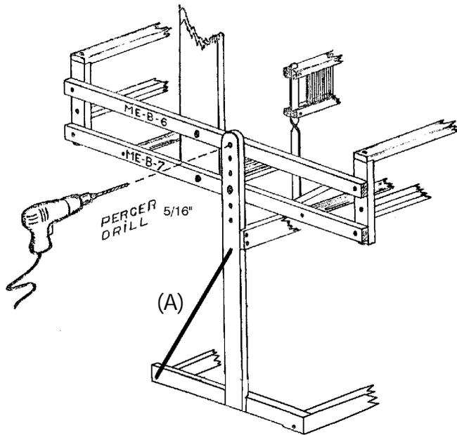
Using the square head screwdriver supplied with loom or a std. philips screwdriver, install the metal post (A) using the 2 screws #12  $\frac{3}{4}$ " already in the uprights.
