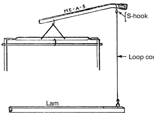
Install the loop cord. Place the S-hook over each lever and insert the other end of the cord in lam's hook. Adjust the lenght by using different hole in loop cord.
