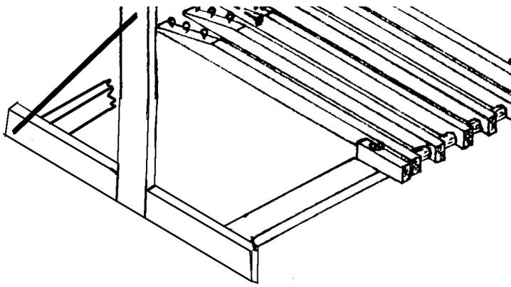
Screw the Upright post to the base using the 4 Carriage bolt  $\frac{1}{4}$ " x  $1\frac{3}{4}$ ", 4 washers  $\frac{1}{4}$ " and 4 square nuts  $\frac{1}{4}$ "
