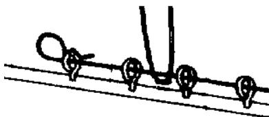
Install the treadle cords trough the lam and treadle hooks. For more information, see book Warp & Weave supplied with the loom.
