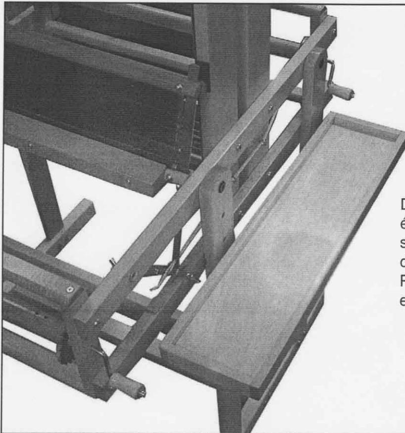
Place the right shelves on top of the squares so it will be as close as possible to the front of the loom but away from the full rotation of the cloth beam crank. Place the opposite side shelve at the same distance to the front.
