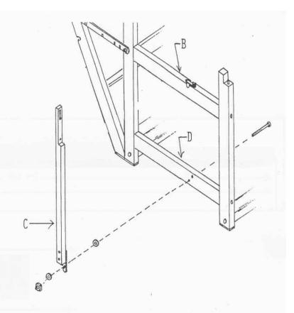
Affix batten swords C to lower lateral cross-members D. Insert the two 5/16 x 21/4" carriage bolts to the **LOWER HOLE**.
