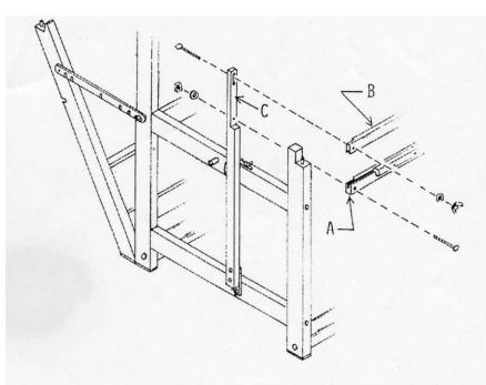
NOTE: When putting the Bolts back in the Batten Sley and the Handtree, the bolts for the Sley go front to back with the nuts in the back, and for the Beater Handtree they go from back to front so the Wing Nuts are in the front.
