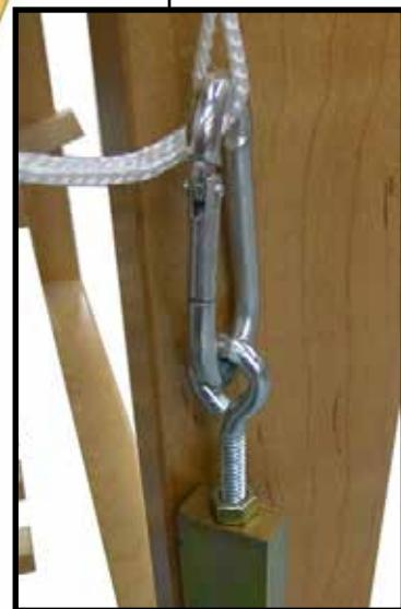
Affix the eyescrews using a 7/64" drillbit to make the pre-drill holes.
