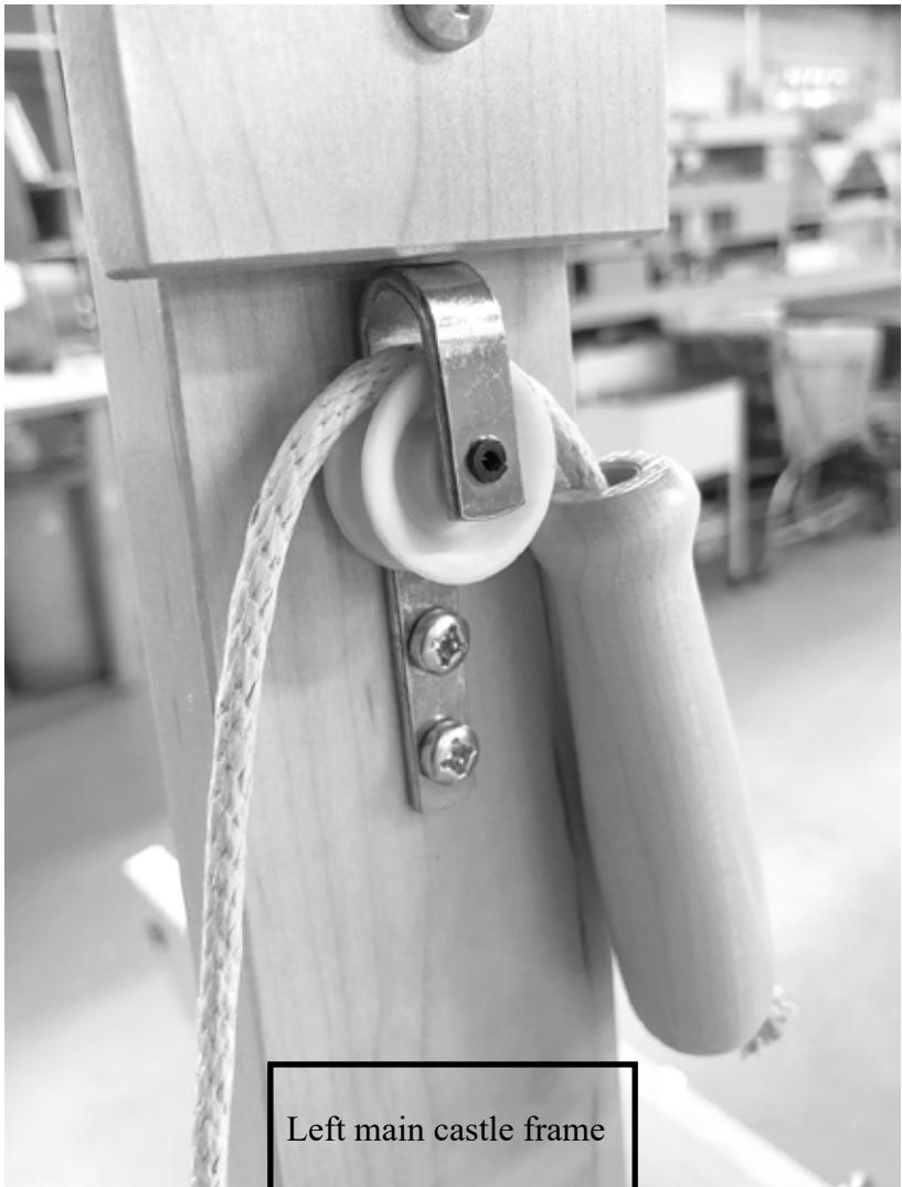
Affix one pulley with plate to the main frame castle using 2 screws no 8,  $\frac{3}{4}$ "
