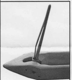
smooth surface Yarns to the coarser Handspuns. A few turns of the Tension Control Key provides micro adjustment for exact Yarn feed. Insert the Key from either side and turn clockwise to tighten, counterclockwise to loosen. It's that simple.
