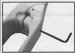
The Pirn Spindle will accommodate a variety of Pirn(Bobbin) bores by inserting a flat screwdriver head under the self adjusting Spindle Spring to increase the diameter or tapping the mid point with a small Mallet to decrease.
