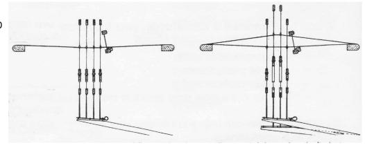
depressed, these shafts will rise while all the other shafts remain stationary. The size of the shed is dependent upon the tension of the warp threads, how many threads there are and the strength of the weaver.
