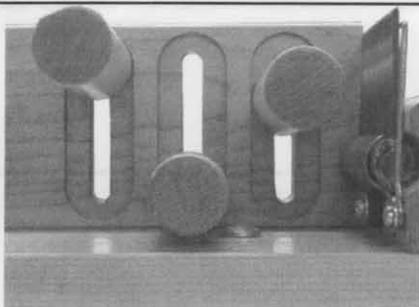
Install the tension box rollers and adjust them for the tension desired. Many configurations are possible.
