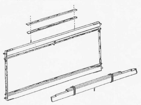
When necessary, to keep shaft down (for a cleaner shed), add weights (1 or 2) on top of the shaft frame.
