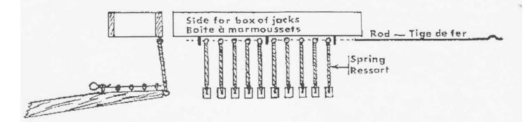
Some looms are equipped with springs to hold the weight of treadles and prevent shafts to raise by the weight of it.
