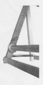
Remove the old pawls of both beams. Affix a new pawl to the bottom beam with a round-head 3/4 screw #12. Make sure the pawl fits perfectly inside the teeth.
