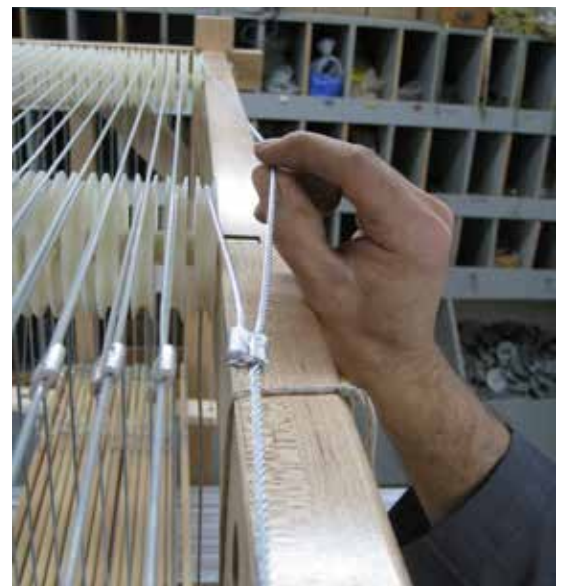
Make sure that the loop sleeves of the cables are parallel to the wood part of the shaft frame to avoid any damage on them.
