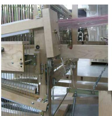
This picture shows a correct adjustment but now make sure the right treadle is app. 1" from the floor.
