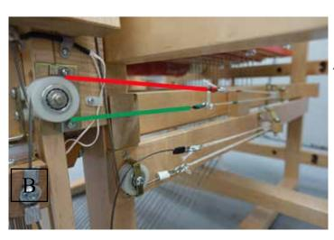
Hold the bottom arm (B) in the closed position (all the way to the nylon stopper)
