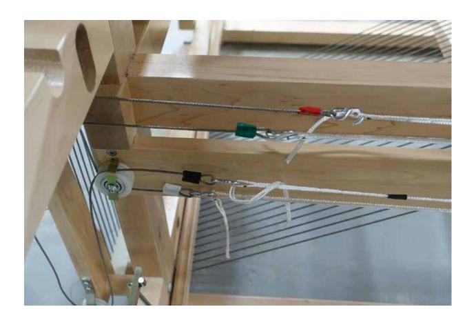
Before threading the loom, make a careful inspection to all the pulleys controlling the arms. (metal cables and loop cords)
