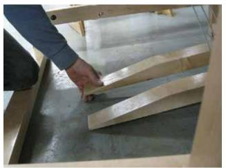
Hold the left treadle app. 1.5" from the floor or place a block 1.5" under it.
