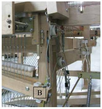
Adjusting the treadle cords without the black marks or checking if the black marks are at the right place.
