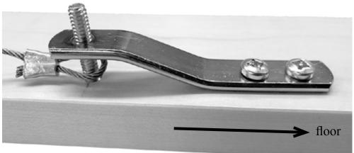
If necassary, use a 7/64" or a 1/8" drill bit to make the predrill hole and affix the strengthening piece using 2x rounded head screw #8, 3/4"
