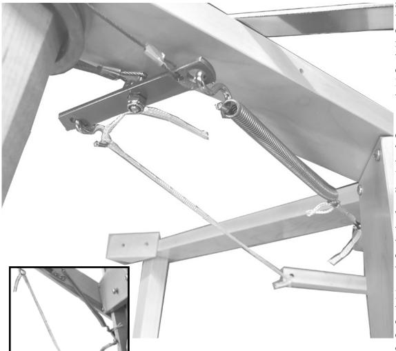
Is it recommended to unhook the spring when winding on the warp (as well as folding the loom)
