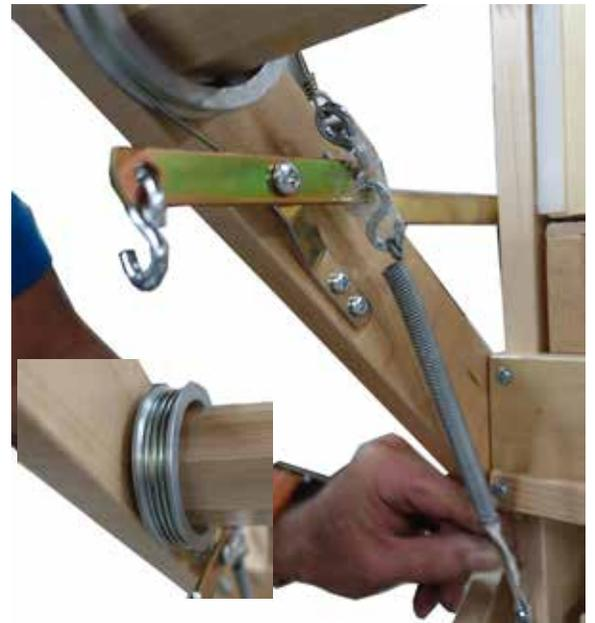
Connect the back lever "S" hook to the brake treadle. Use the black mark as a starting point.
