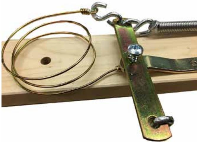
Use the screw no 12, 1 1/4" to install the lever, strengthening piece and brake circle assemble like in this picture.
