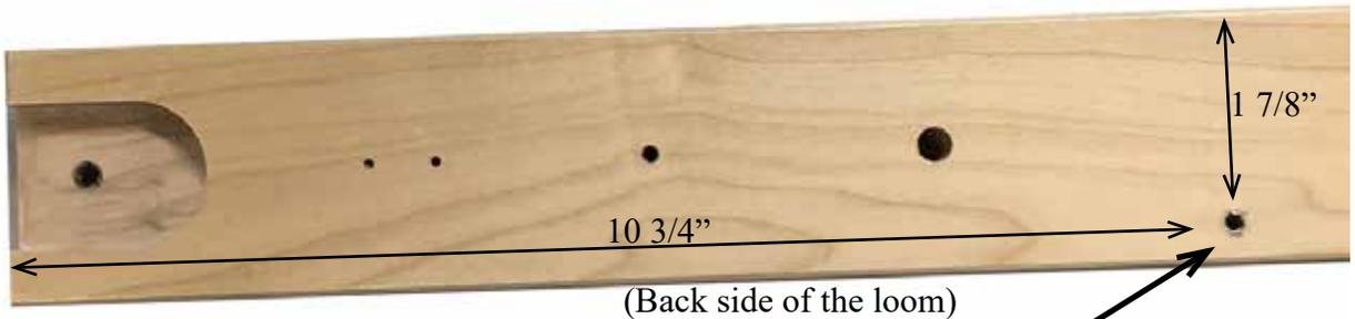
Make a pre-drill hole in the post following this plan. Use a 11/64" or a 3/16" drill bit.
