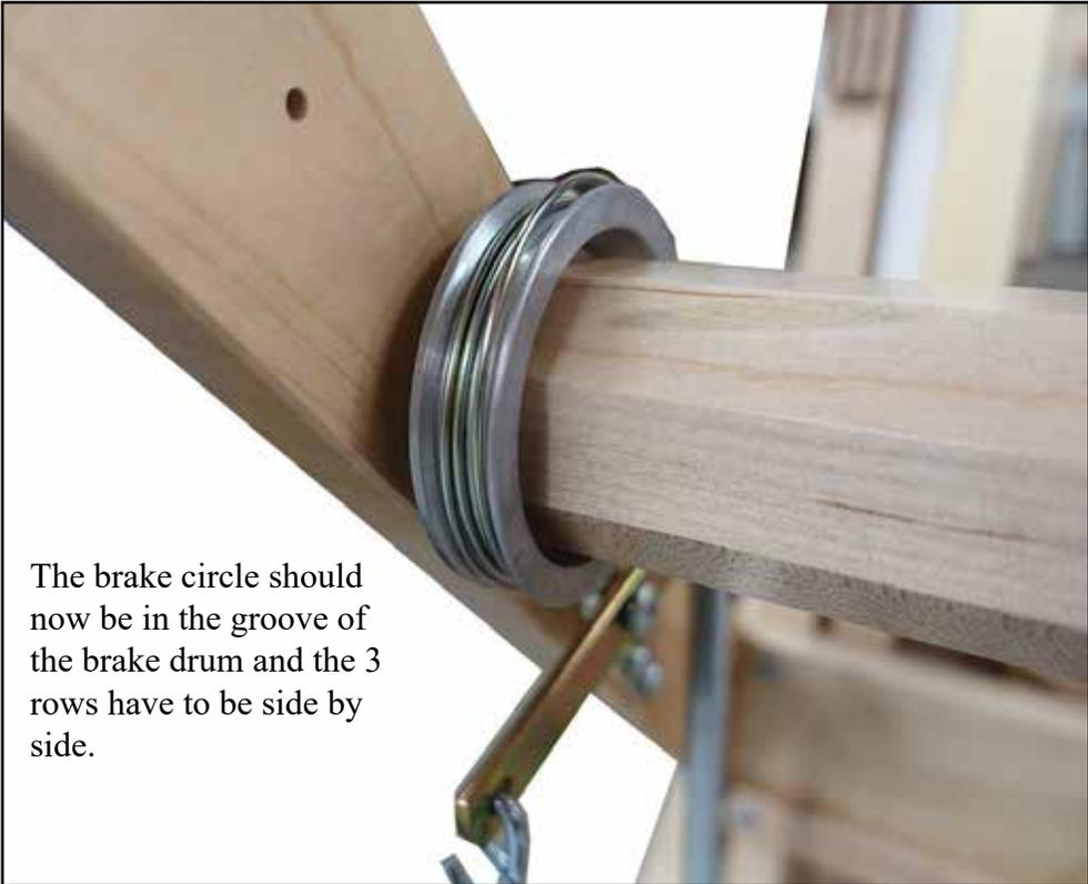
The brake circle should now be in the groove of the brake drum and the 3 rows have to be side by side.
