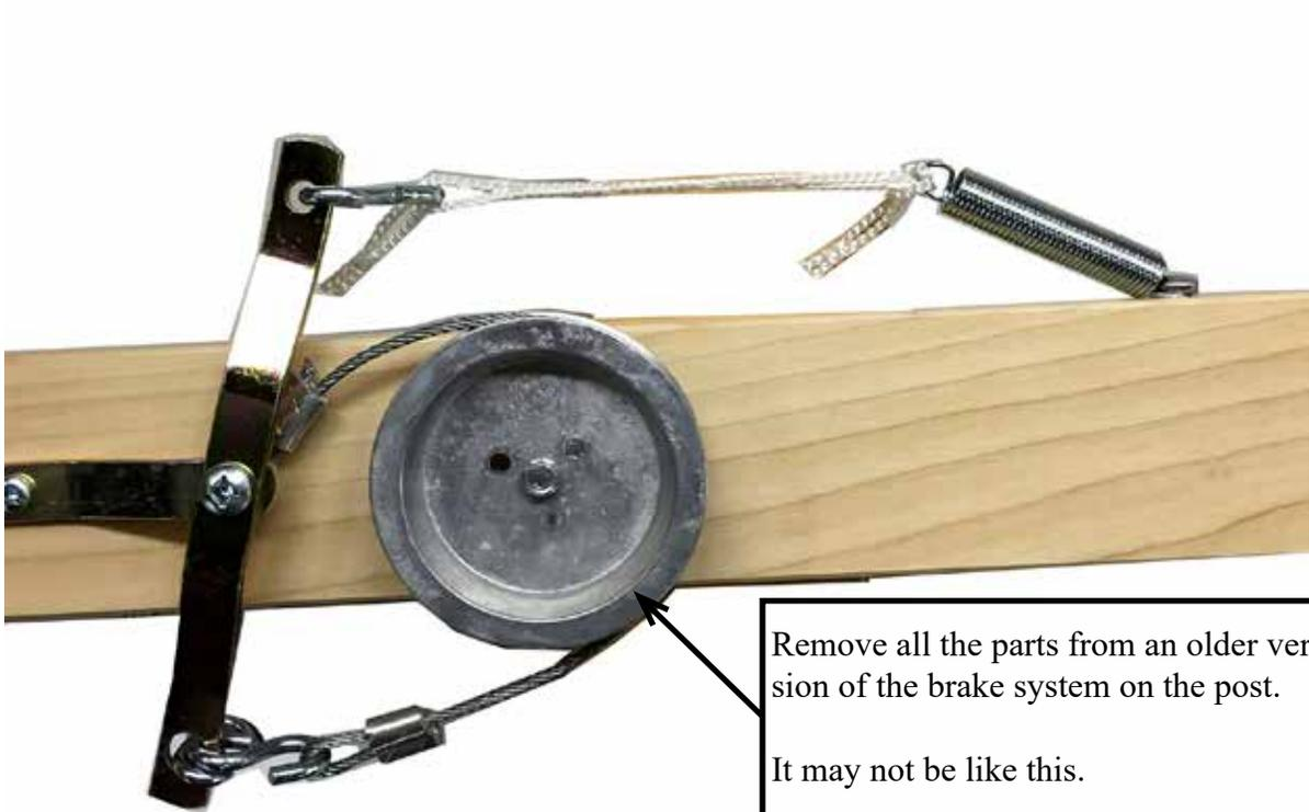
Remove all the parts from an older version of the brake system on the post.
