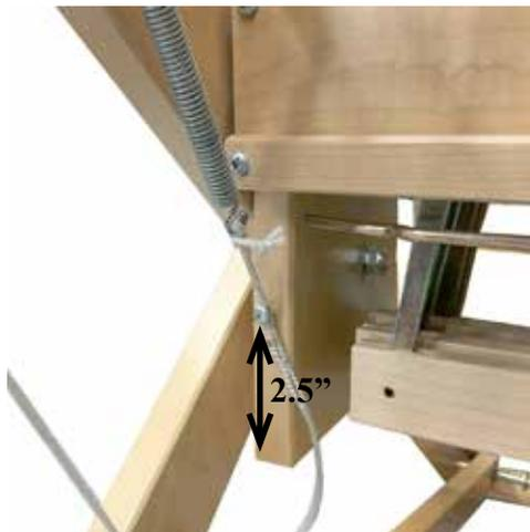
Use a 7/64" or a 1/8" drill bit to make this pre-drill hole to the centre of the right-hand side uprights (in the back of the upright)
