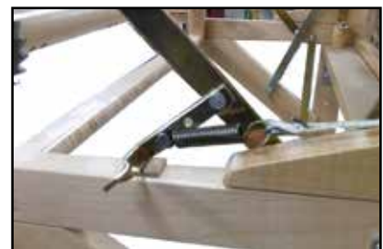
Brake lever closed to tighten the brake cable.
