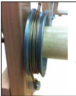
Brake assembly with brake circle. Make sure it is properly in place.
