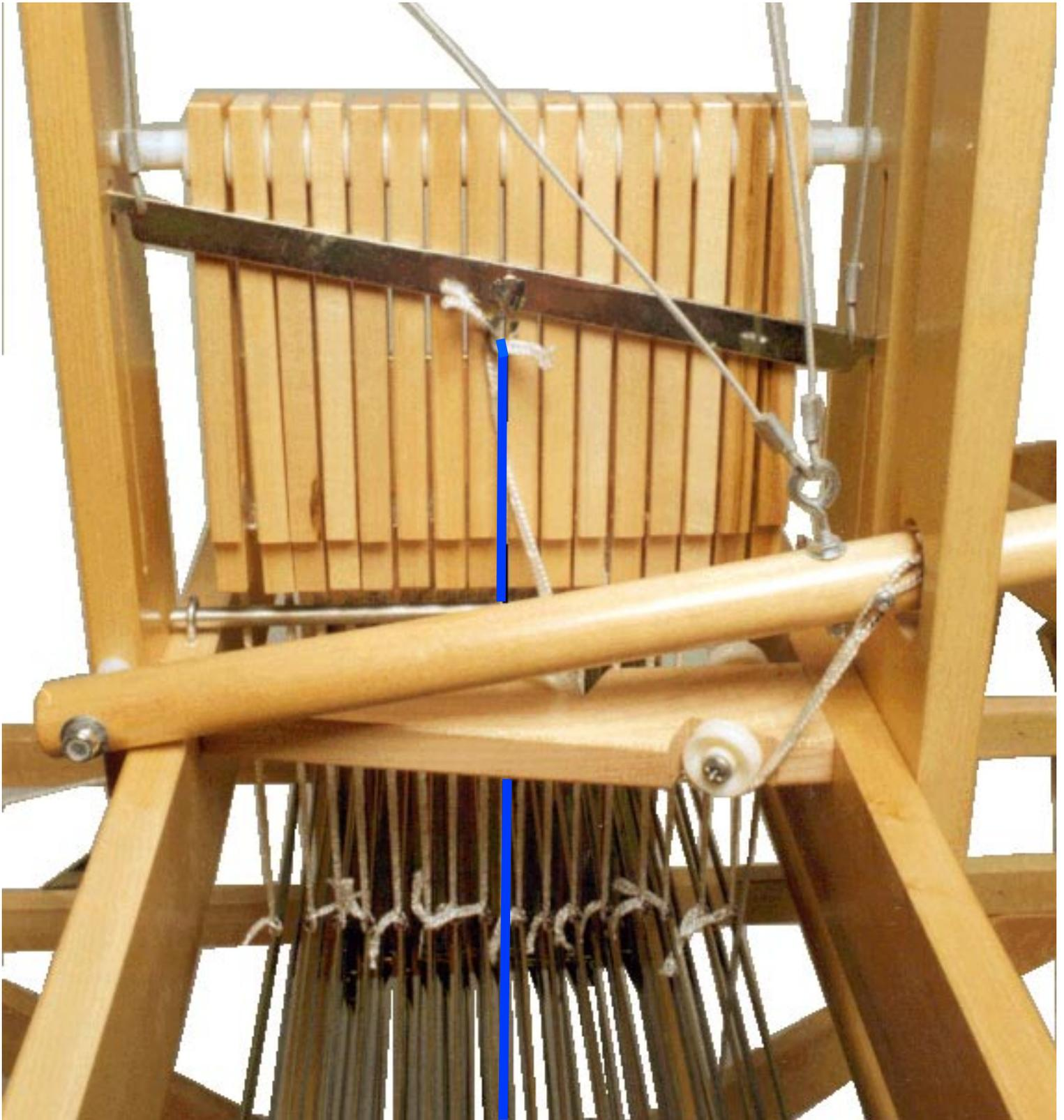
Install the loop cord joining the screw hook of the left treadle and the hook under the knife, threading it between the shaft frames. Adjust the length so the knife is at the low position when the left treadle is depressed.
