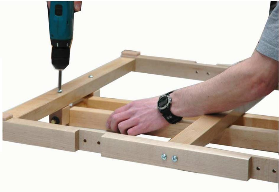
Assemble the 4 uprights to the base using the carriage bolts ¼", 1¾", the square nuts and the washers.
