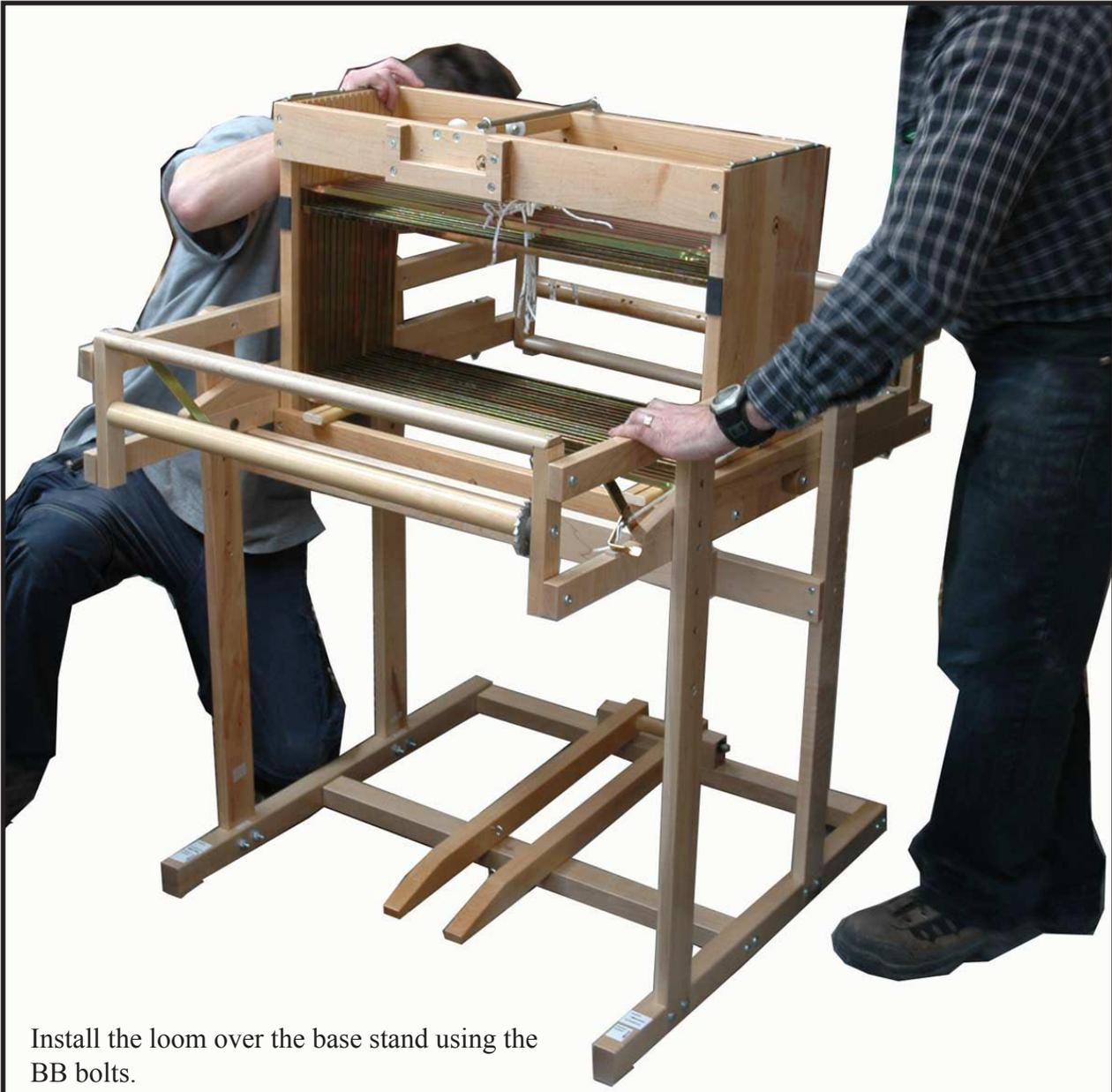
Install the loom over the base stand using the BB bolts.
