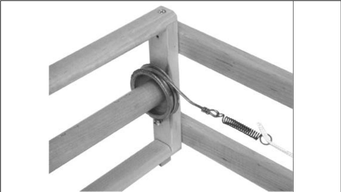
Adjust the height of the reed so the bottom warp threads just touch (or are just a little lower than) the shuttle race when the shed is open. Shed should be at least 1½". If the shed is smaller, you probably weave too close to the reed and (or) the tension on the warp is too high.
