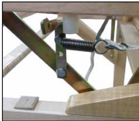
Move it up to release the brake.
