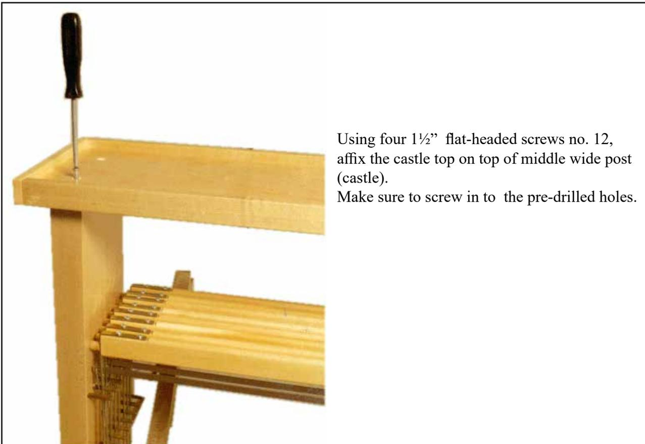
Using four 1½” flat-headed screws no. 12,
