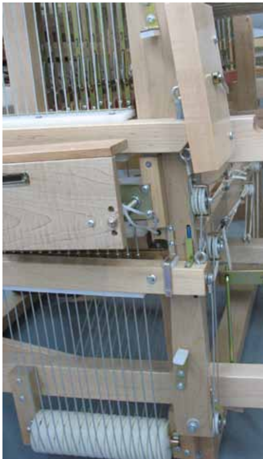
CLOSED SHED WITH LITTLE PRESSURE ON THE LEFT TREADLE: The left treadle is near the floor and there is almost even tension on all the loop cord treadle cables.
