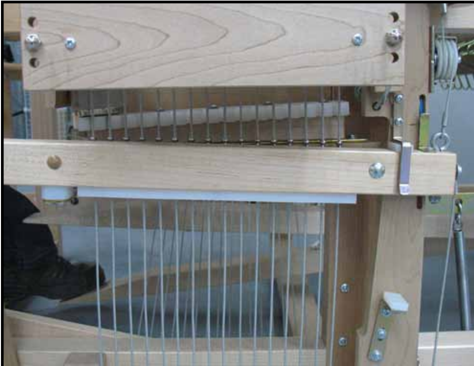
CLOSED SHED WITH LITTLE PRESSURE ON THE LEFT TREADLE: All lower balls out of the fork and lower than the fork
